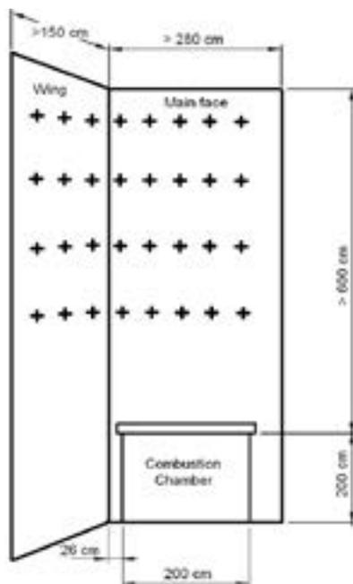
Picture 1 – Configuration of the to façade test sample according to BS 8414-1
