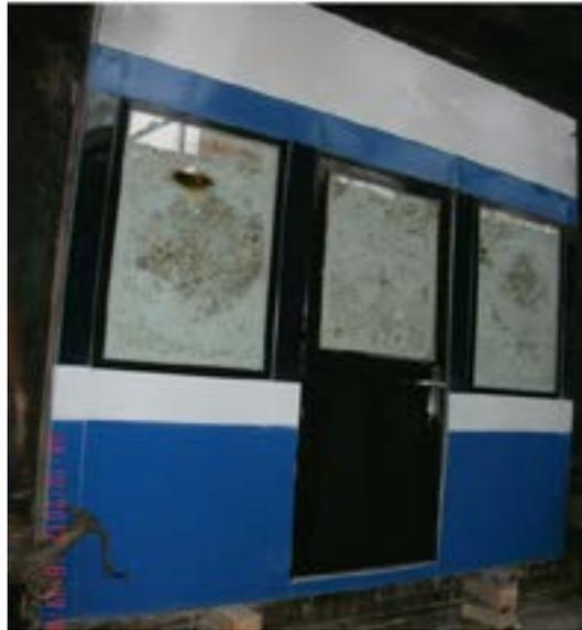
Photo 1 - Model of the end glazed partition after the fire tests on NPB 109-96 (photo V.O.Bulatov).
