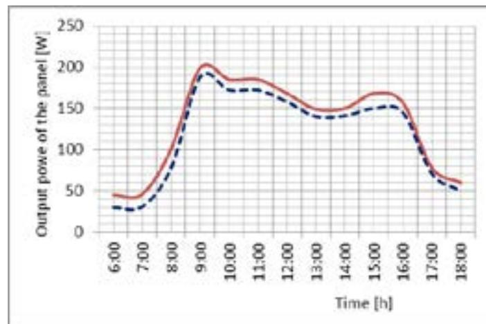
Figure 8. The dependence of the power from the solar radiation intensity with clean (solid line) and dirty panels (dotted line) in cloudy weather
