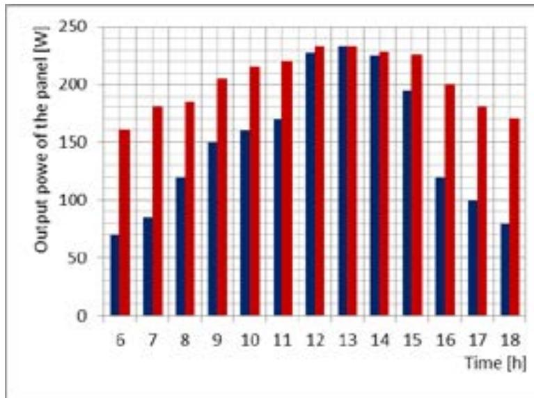
Figure 10. Illustration of the efficiency of the fixed (blue) and moving (red) photovoltaic panels during the day
