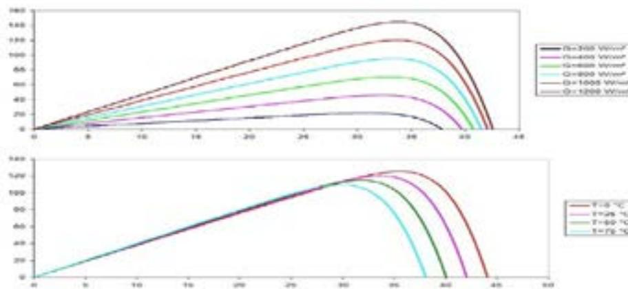
Figure 3. P-V panel characteristics in six different intensities of solar radiation [2]
