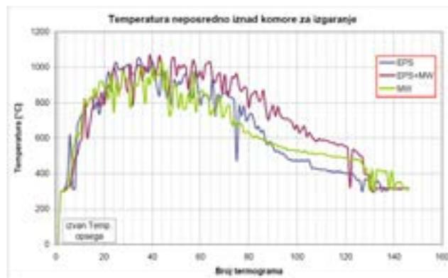
Temperature 125 cm above the combustion chamber
