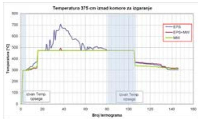
Figure 1 - Distribution of temperature at different heights of samples façade
