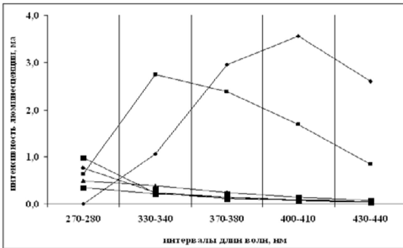
Figure 1. – Coding of rated luminescence spectrums of grassy bio-mass extracts, grown on the soil with different types of oil pollution.
