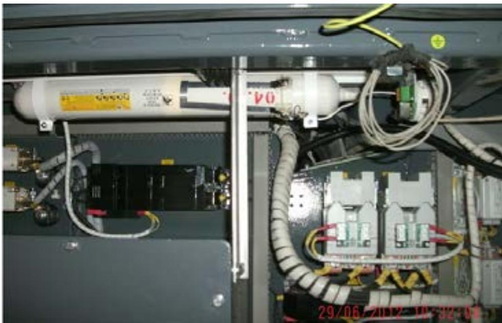
Photo 5 – Self-activated powder extinguisher OSP-1 and the «Fire detector» (IP101-V, located to the right of OSP-1) in the undercar space, cover is opened. (photo V.O.Bulatov).
