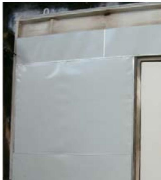
Photo 2 - Model of the partition between the cabin and the control after the fire tests on NPB 109-96 (photo V.O.Bulatov).
