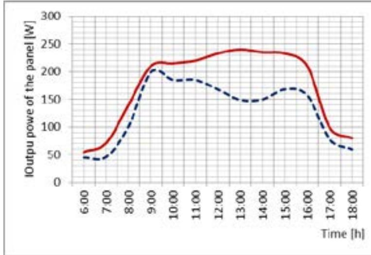
Figure 9. The dependence of the power from the solar radiation intensity with clean panel in sunny (solid line) and in cloudy weather (dotted line)
