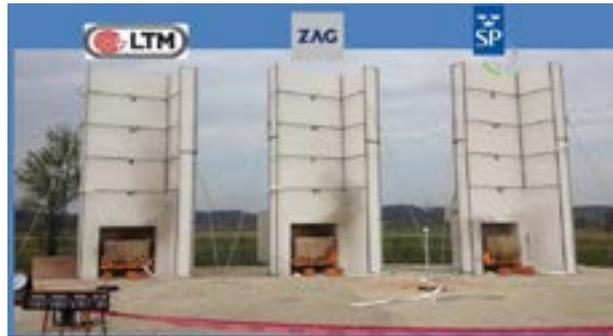
Picture 2 – Layout of façade samples, during the fire test
