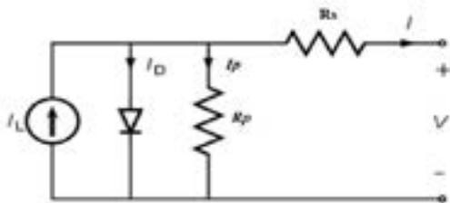
Figure 1. One diode model of photovoltaic cells [1]
