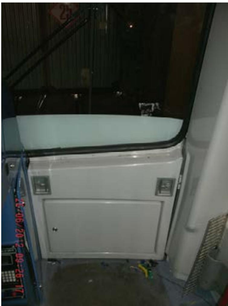
Photo 7 - Exit on concrete track through the door located in the cab of the train “Neva” (photo V.O.Bulatov).
