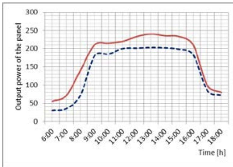
Figure 6. The dependence of the power from the solar radiation intensity with clean (solid line) and dirty panels (dotted line) in sunny weather
