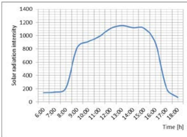
Figure 5. The change of solar radiation intensity in sunny weather
